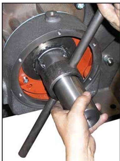
Pins key for Nut mounting (see Technical data sheet for each model)
