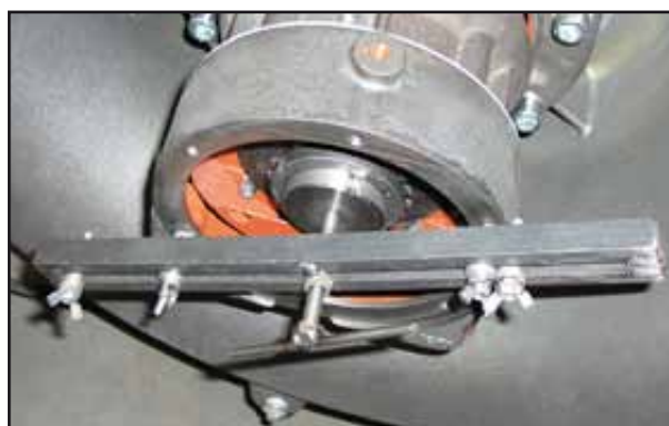
Tool for maintaining rotor in position during bearing change. (see Technical data sheet for each model)
