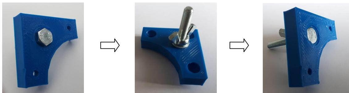
Figure 2: Install hexagon bolt in base block
