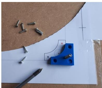
Mount the base blocks as precisely as possible at the location indicated by the template, but only screw them to the mounting point marked in red. So you **don't put the second screw** in yet. Tighten the first screw so that the block clamps well but you can still turn it with some force. Do this for all 4 blocks.<sup>2</sup>
