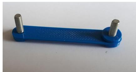
Fig. 3: Hexagon bolts in locking plate
